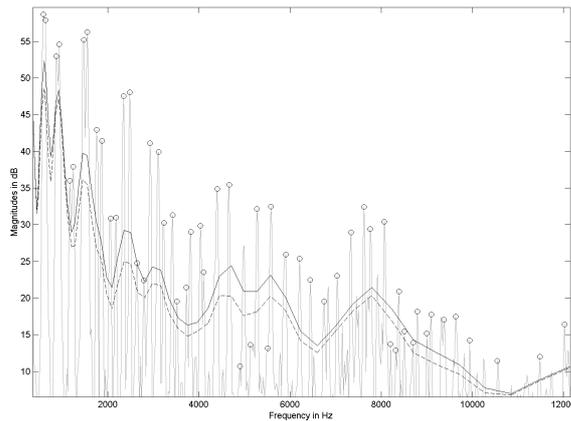
Figure 3. Spectrum of a piece of two-pitchpipe-mixed signal (dotted line), circles indicate components that cause excess masking, masking threshold without excess masking (dashed line), with excess masking (solid line). The masking thresholds are lifted parallel upwards for better visibility.
